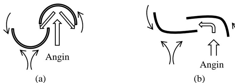
Gambar 2.13 (a) Rotor Savonius U, dan (b) Rotor Savonius L (Soelaiman, 2006)
