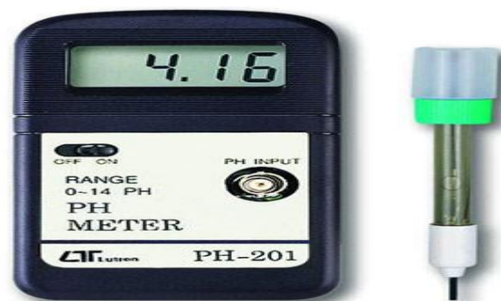
Gambar 2.11 pH Meter Digital
