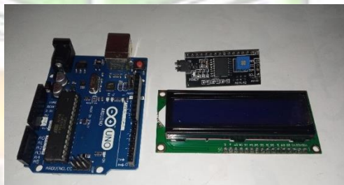
Gambar 4.7 Perangkaian LCD I2C
