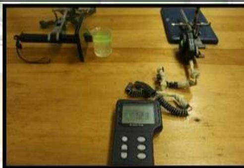
Uji Kejernihan Sampel Air Pada Inlet Filter
