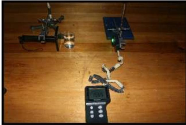
Uji Kejernihan Sampel Air Pada Outlet Filter
